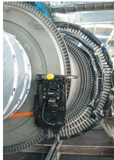
SPM mounted on a turbine
